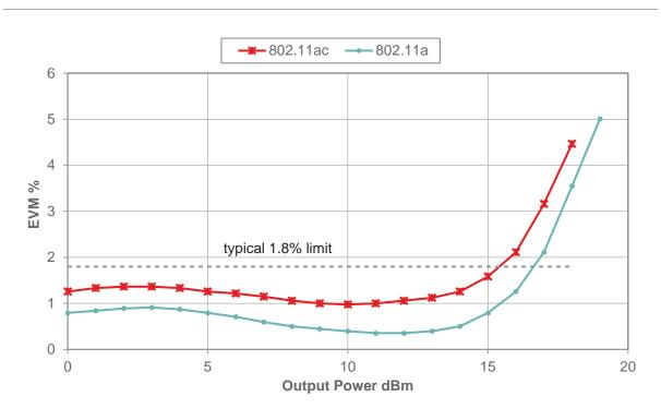
Figure 4 • 5 GHz WLAN PA EVM
