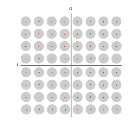
Figure 2 • 256 QAM Constellation Diagram
